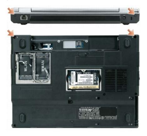
NOTICE: When removing the display assembly, carefully unthread the Mini-Card antenna cables through the computer base and ensure that the plastic protectors—if present—remain on the individual cables.
