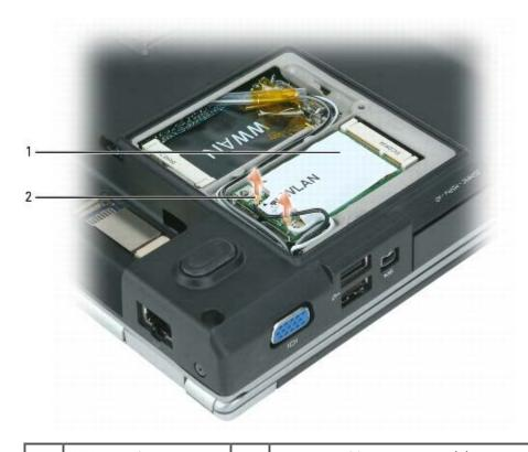
1 WLAN card 2 antenna cable connectors (2)
